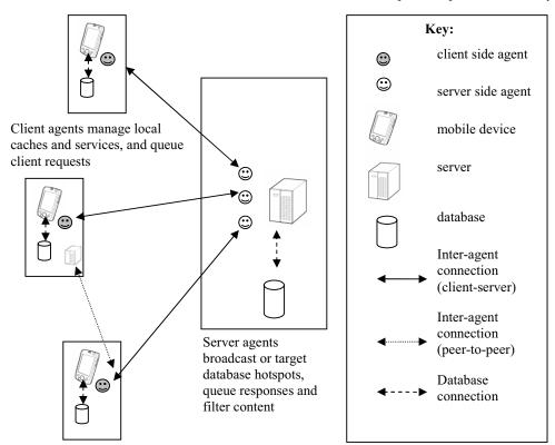
Figure 1. Components of a mobile architecture
