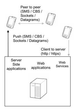
Figure 3. Components of a mobile application architecture
